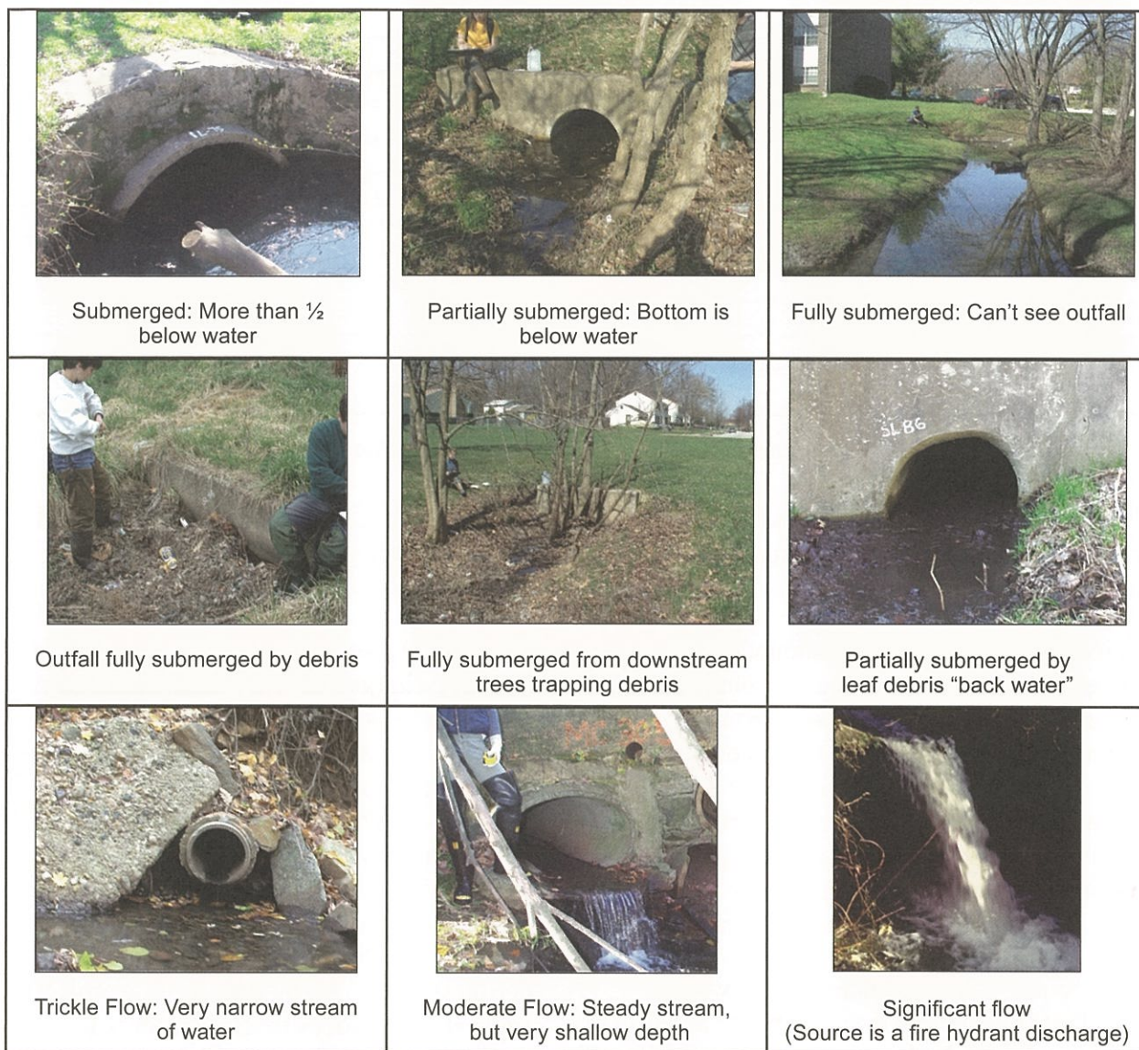
Figure 28: Characterizing Submersion and Flow
