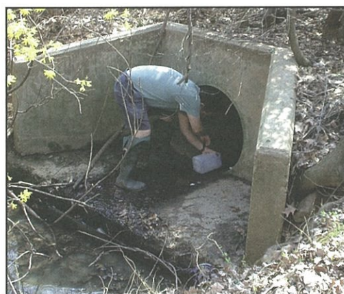
Figure 30: Measuring flow (as volume per time)
