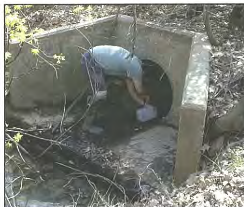
Figure 30: Measuring flow (as volume per time)
