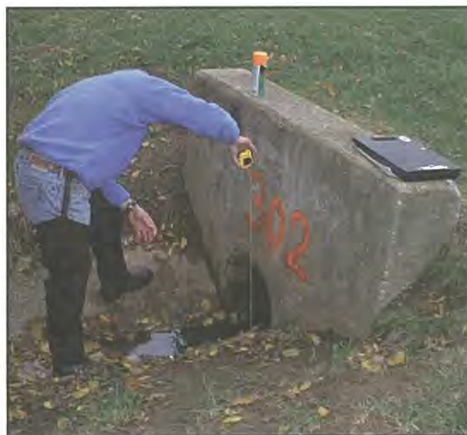
Figure 27: Measuring Outfall Diameter
