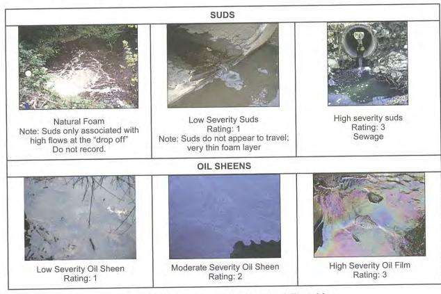
Figure 35: Determining the Severity of Floatables
