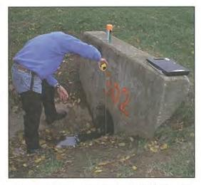
Figure 27: Measuring Outfall Diameter
