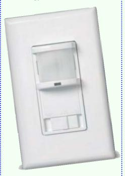
the Doppler principle. These sensors produce low intensity, inaudible sound and detect changes in the sound waves it produces that are caused by motion, such as walking into the room, reaching for a telephone, or turning in a chair. They are volumetric in nature and are not line-of-sight dependent. Since they fill the space with these sound waves, they are excellent in bathrooms with stalls, enclosed hallways, or other oddly shaped
